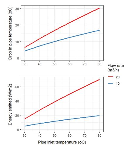
Heat pipe energy is emitted as a combination of radiant and convective heat. We denote the proportion of long-wave radiation  $p_{pipe}^{lw} \in [0;1]$  and, assuming that it is radiated equally down- and upwards, we get
