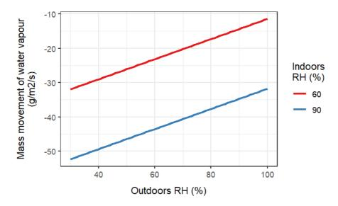
The cooler outdoors air can hold only little water. Hence, ventilation is an effective means of lowering indoors humidity. The effect is larger with more humid indoors. The flux of water vapour is negative because water is lost from the greenhouse. Since the humid indoors air holds latent heat originally captured by transpiration, ventilation also functions as an indirect route of venting excess heat.
