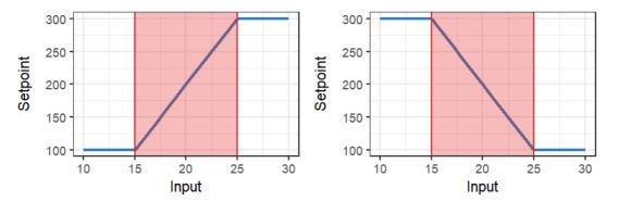
Such proportional setpoints are defined by their range ([100; 300] on the y-axis above) in response to an input threshold (15 above) and a threshold band (10 above). The response can be increasing (left figure) or decreasing (right figure).
