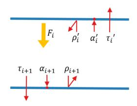
Our first aim is to find out, how much of the downwards radiation from the upper layer  $F_i$  (W/m<sup>2</sup>), e.g  $F_i^{sw}$ , is absorbed by the lower layer? If we denote the *net* absorption from above  $\hat{\alpha}_{i+1}$ , we immediately have
