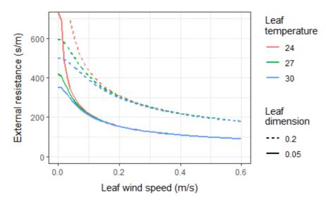
Both  $\ell$  and u are difficult to estimate.  $\ell$  should be smaller for smaller leaves. u should increase with the greenhouse ventilation rate (or if rotors are running) and decrease with  $L_{ai}$ , as a denser canopy will reduce the average wind speed at leaf surfaces.
