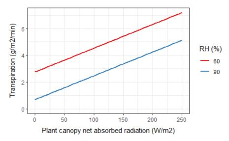
Obviously, transpiration is larger in a drier climate and it increases with the absorbed radiation. Note that leaf temperature (previous figure) too increased with absorbed radiation. This means that the increase in transpiration with increased absorbed radiation was not sufficient to keep leaf temperature constant; that would have acquired an even higher transpiration.
