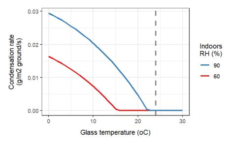
The vertical line at 24°C highlights that at high indoors humidity (90%), just a slightly cooler glass will accumulate condensation. The condensation rate is in the same range as transpiration, e.g., at 90% humidity and a glass temperature of 10°C, the condendation rate is  $0.02 \text{ g/m}^2$ /s (read off the figure) giving  $1.2 \text{ g/m}^2$ /min.
