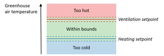
The humidity is controlled indirectly through manipulation of the temperature setpoints, e.g., if it is too humid then the ventilation setpoint is lowered.
