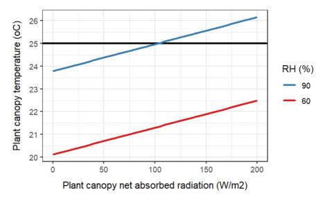
Clearly, a high air humidity works against plant transpiration and leads to a higher leaf temperature, even above the ambient temperature of the greenhouse: Relatively cool leaves are a sign of a sound microclimate.
